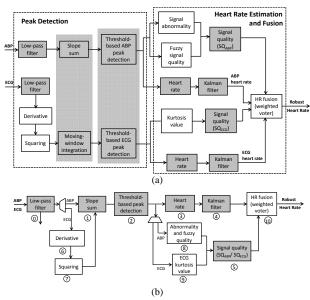
Fig. 1. Robust heart rate estimation flow
