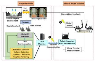
Fig. 2. Hardware-in-the-loop Surgical Simulator Architecture.
