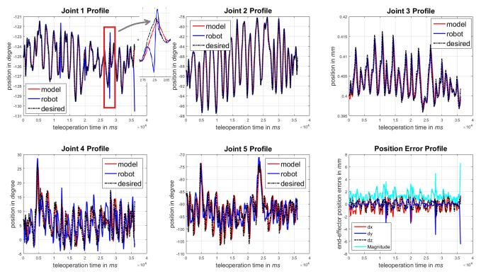
Fig. 4. Robot and model trajectories during fault injection is enabled (with teleoperation scaling factor of 0.1)
