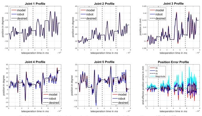
Fig. 3. Comparison of the model and robot running data (up to 5 joints), and end-effector position error of  $(2.43 \pm 1.72)mm$
